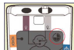
Figure 2: The GSI indicates 75% good quality
